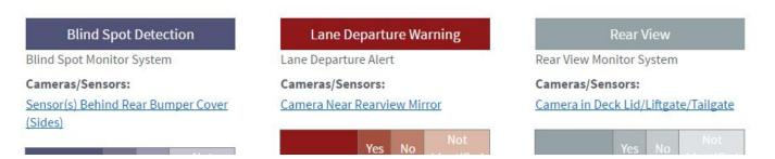
Having this information easily accessible during the damage analysis/blueprinting process can save valuable time and allow for more accurate damage assessments and repair plans. Knowing early on that the vehicle will have to undergo an aiming/calibration procedure will reduce surprises later in the repair process — or even worse, after the vehicle is delivered back to the customer.
