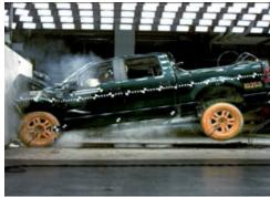
The bumper beam, which lies unseen beneath the decorative plastic bumper cover, plays a critical role in auto safety. In a frontal crash, the bumper beam is the first structural part to suffer the impact and initiate vibrations through the vehicle body. Those vibrations are ultimately picked up by sensors, which determine whether the air bag should be deployed or not, and how quickly.
