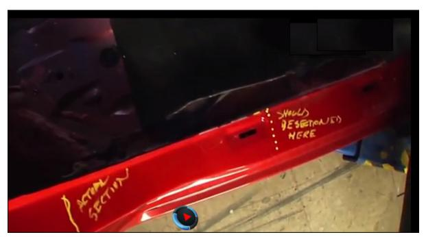
See some of the issues that can be uncovered in a post collision repair inspection. (Video-Pack Brothers Collision Center and AP Media)
